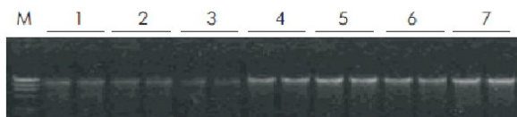
Figure 1. Purified genomic DNA from 7 different water sources was isolated with the E.Z.N.A. ® Water DNA Kit. DNA was extracted in duplicate from water samples as follows: sample 1 from 20 L tap water, sample 2 from 5 L air conditioner water, sample 3 from 3 L spring water, sample 4 from 2 L sanitary waste water, sample 5 from 5 L lake water, sample 6 from 6 L pool water, and sample 7 from 3 L industrial sewage water. Genomic DNA (30% of total purified DNA) was analyzed on a 1% agarose gel to demonstrate yield and quality of the DNA. M: Lambda Hind III DNA Marker.
